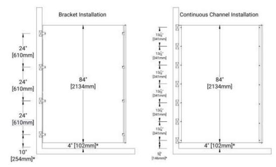
Note: Floor to ceiling pilasters to be installed with an AFF of 4 1/2" (114mm).
