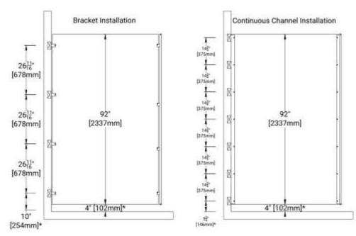
Note: Floor to ceiling pilasters to be installed with an AFF of 4 1/2" (114mm).
