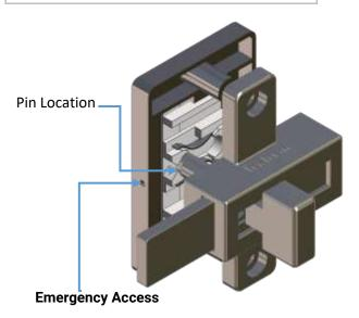
Insert a pin or Allen key 5/64" in diameter or smaller to push open the latch.
