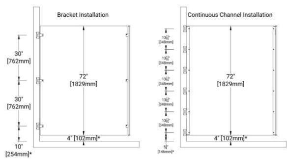
Note: Floor to ceiling pilasters to be installed with an AFF of 4 ½" (114mm).
